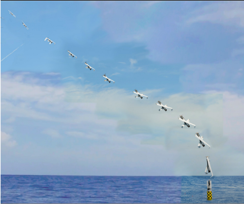
'Upward-falling payloads', sea-launched UAVs (right, US Navy); Co-operating drones (left, GRASP Lab UPenn)
